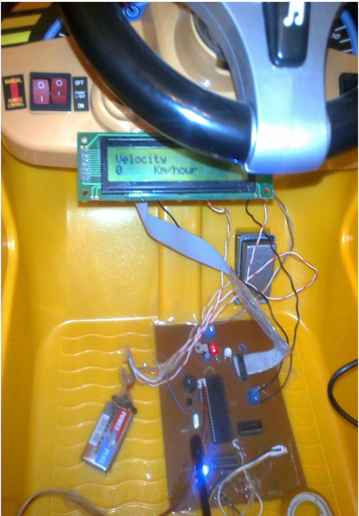
Figure 4-7: Vehicle LCD and Main Controller
