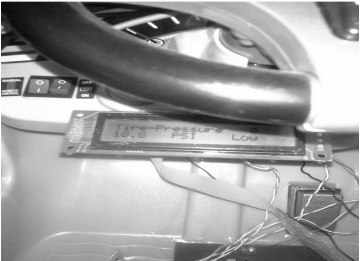
Figure 4-8: Tyre Pressure on LCD
