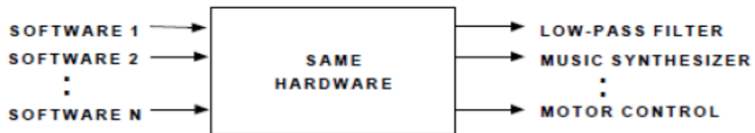
Figure 3.4: Multitasking through DSP
