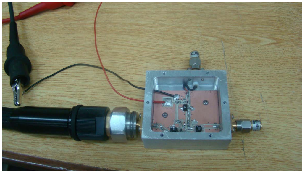
Figure 6-14: Setup for Measuring VSWR
