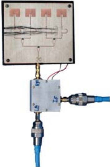
Figure 9-1: Complete Beamformer Structure
