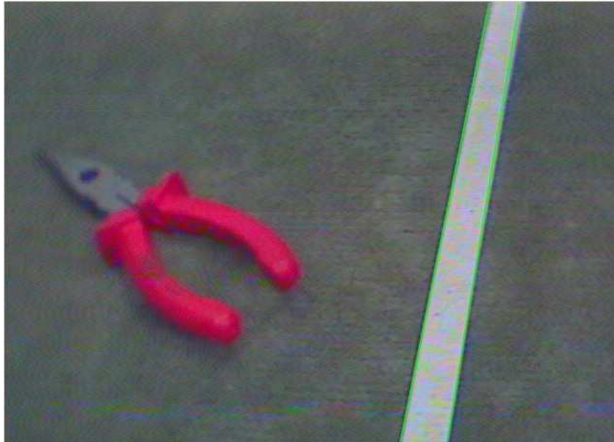
Figure 4.4e Hough Line Transform applied to the binary frame. The edges are marked by the green lines.
