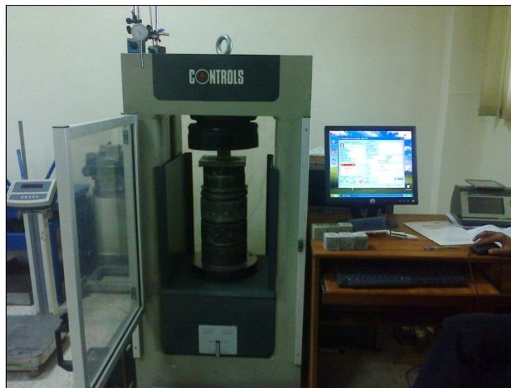
Figure 3.7: Compression machine used for compressive strength analysis of mortar specimen
