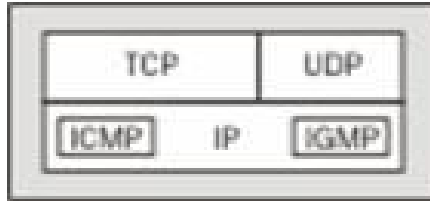
Figure 6: Internet Control Message Protocol in OSI Model
