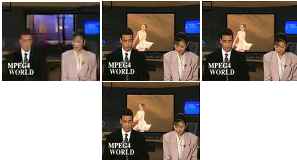
Figure 6.3: Frame number 137 (left most) transmitted over STBC and frame number 138 , 139 and 140 (second, third and fourth) transmitted over SM at an SNR of 28dB
