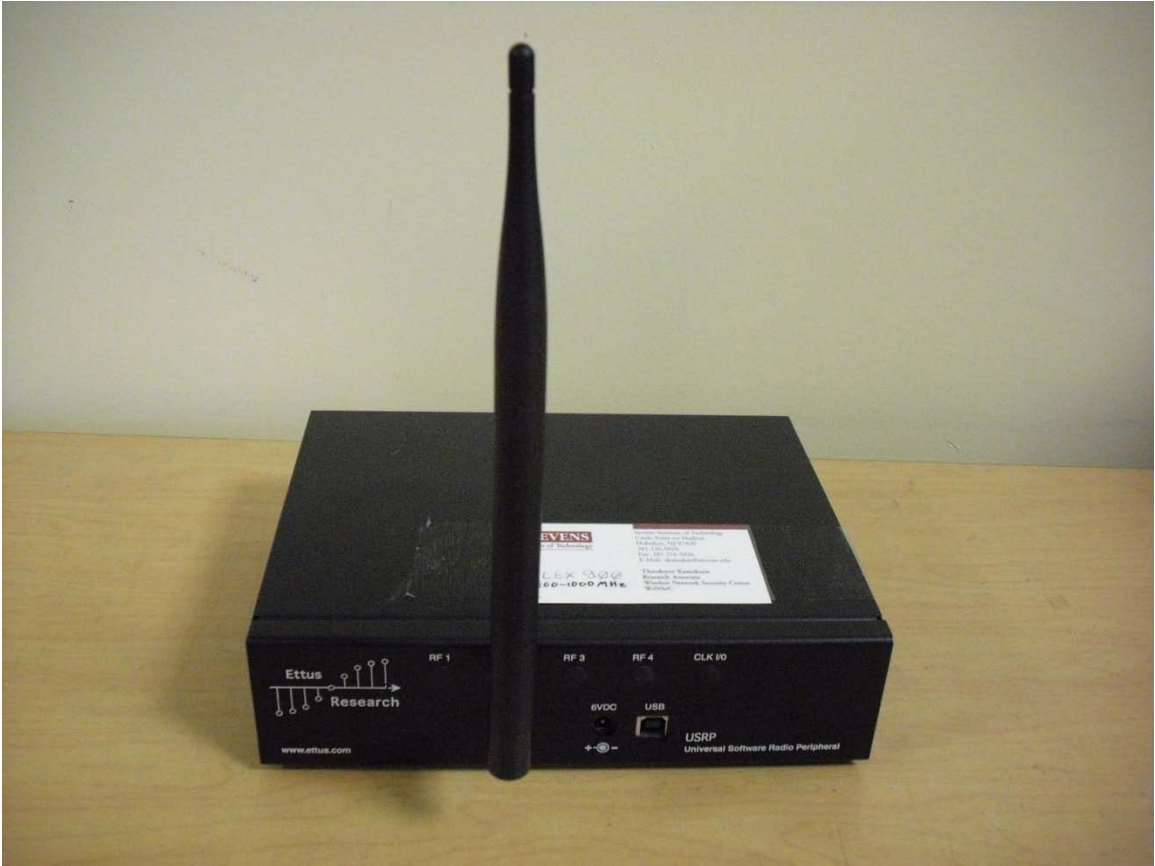
Figure 15: USRP with front end
