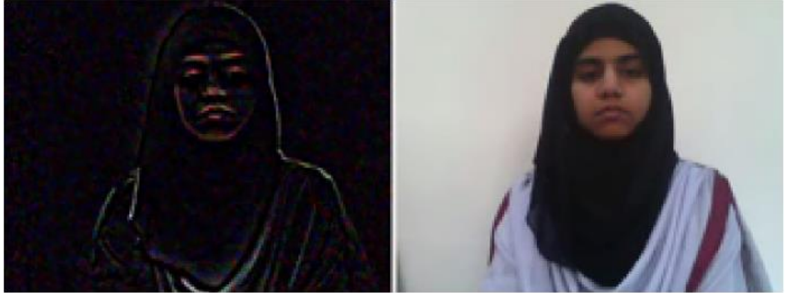
Figure 10: Original (on the right) and Laplacian pyramid combined with IIR filter (on left) frames
