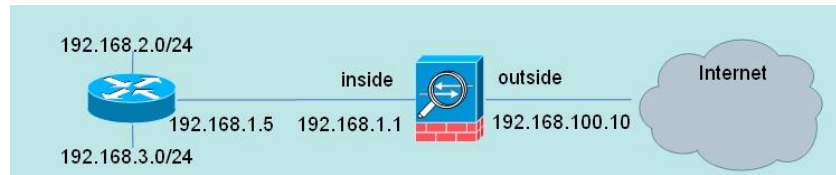
Figure2.5: Firewall in Routed Mode
