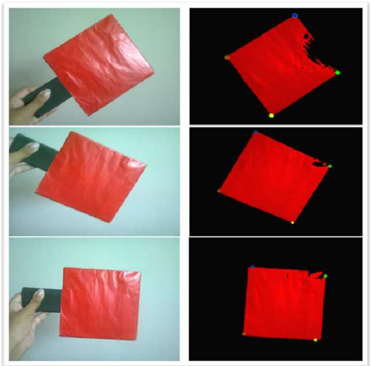
Figure 5-11: Corner Detection with three basic orientations
