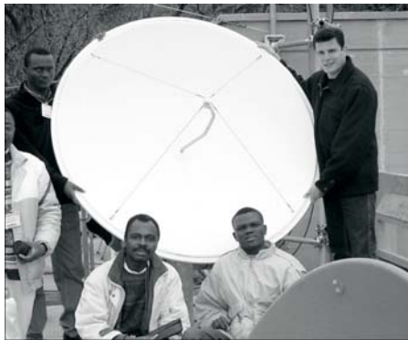
Figure 2.6: A 3.2 GHz Parabolic Dish Antenna
