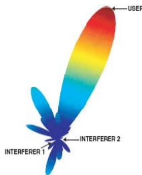
Figure 4.10 Adaptive array coverage: A representative depiction of a main lobe extending toward a user with nulls directed toward two co-channel interferers.
