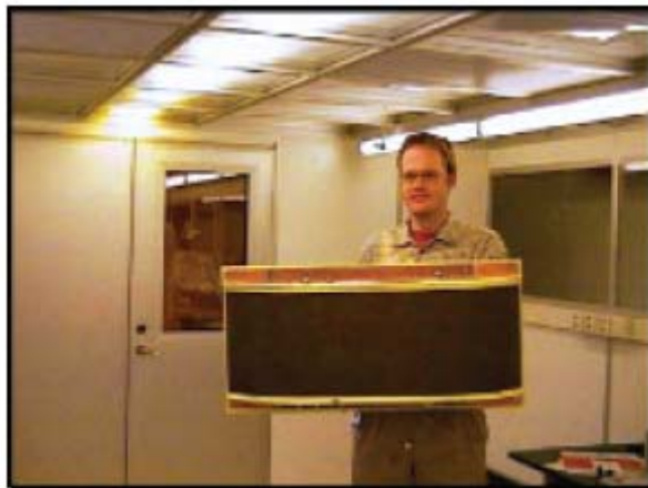
Figure 4.19: Picture of an eight-element array antenna at 1.8 GHz. (Antenna property of Telia Research AB, Sweden) [14].
