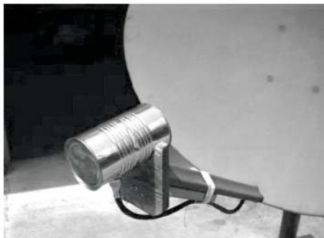
Figure 2.5: A Horn Antenna made out of can
