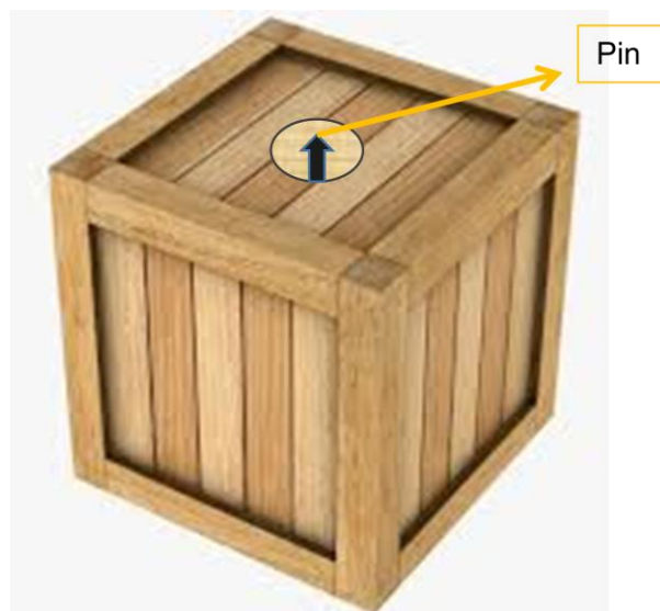
Figure 3.5- Tactile Stimulator. The pin is elevated through the hole and touches the index finger of the participant.
