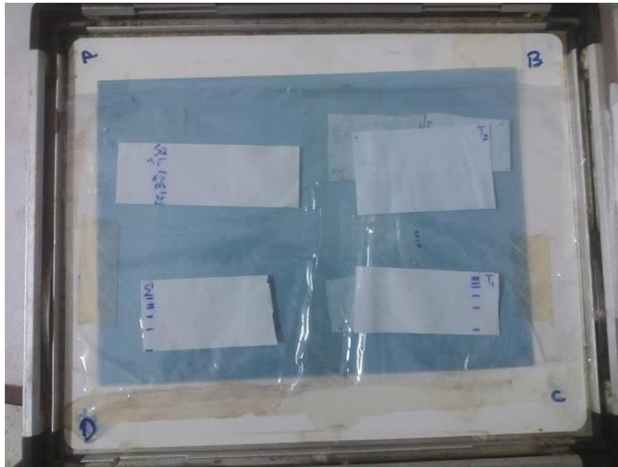
Figure 3.10: Setting NC Membrane in X-Ray Cassette
