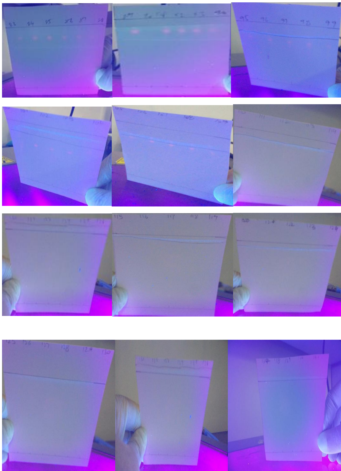
Figure 8 Chromatogram of fractions 83 to 141 on TLC using 15% methanol in EtOAc
