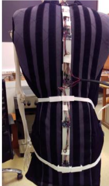
Figure 9 Wearable spine monitoring system with flexible straps (21)
