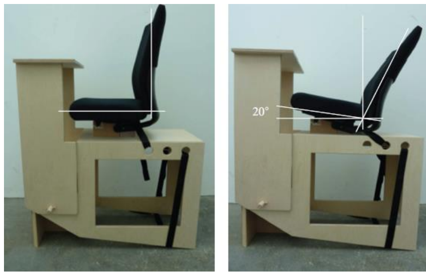
Figure 4 MRI Compatible chair to study posture during different sitting positions (11)
