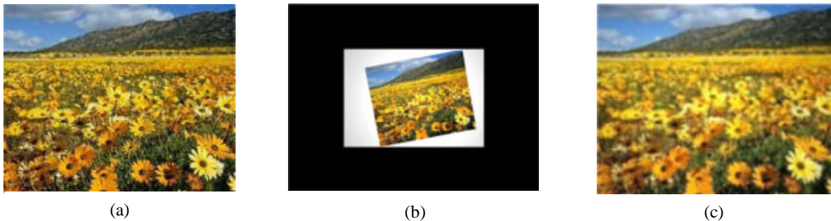
Figure 3-1: Images of projector domain to camera domain conversion process (a) Projector domain image, (b) Camera domain image, (c) Domain converted captured image
