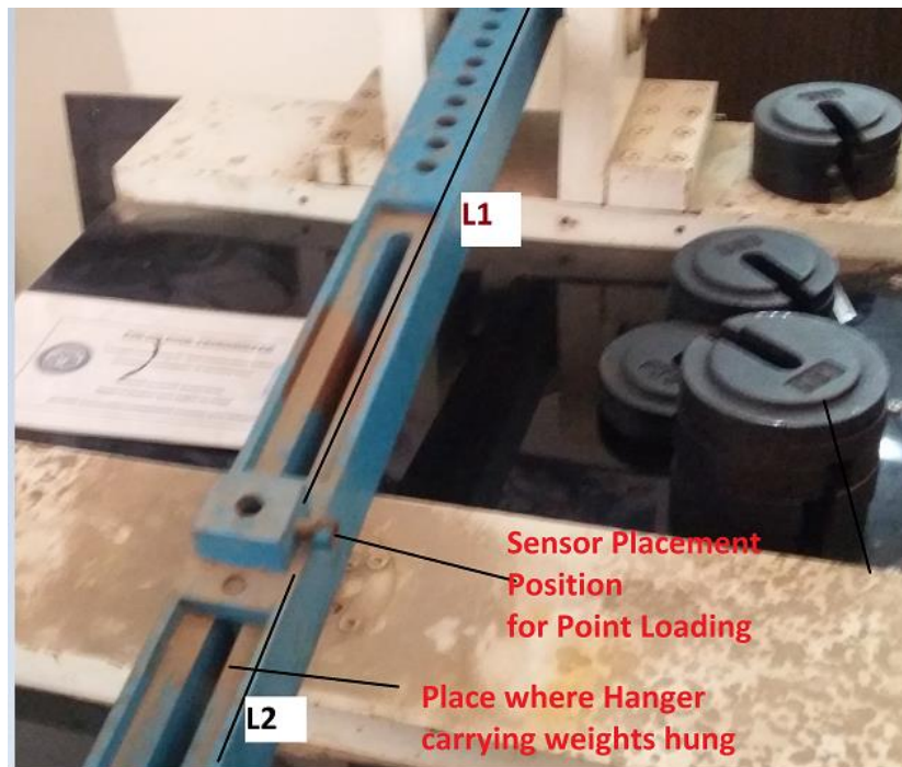
Figure 15 Sensor Calibration Method
