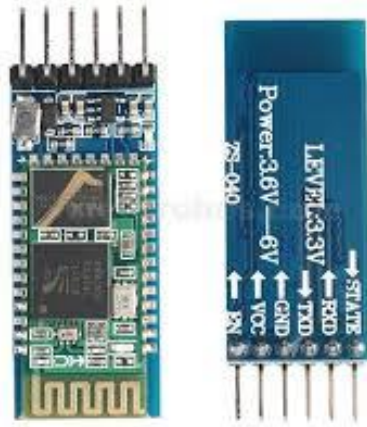
Figure 4: Bluetooth Module HC-05
