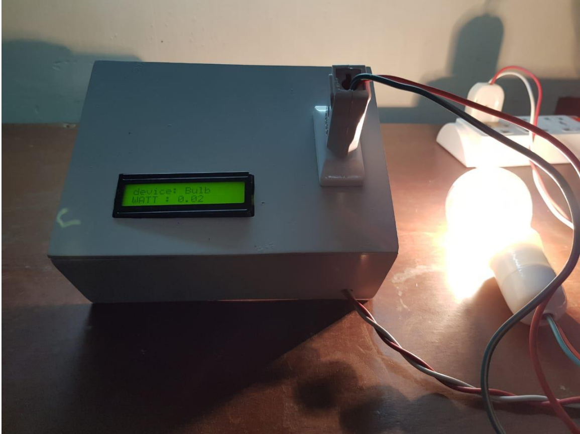
Figure 4-6: Smart Sense Switch Board
