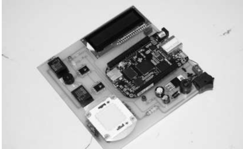
Figure 17: PCB of Image Processing System
