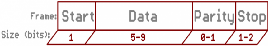
Figure 10: Asynchronous Serial Frame
