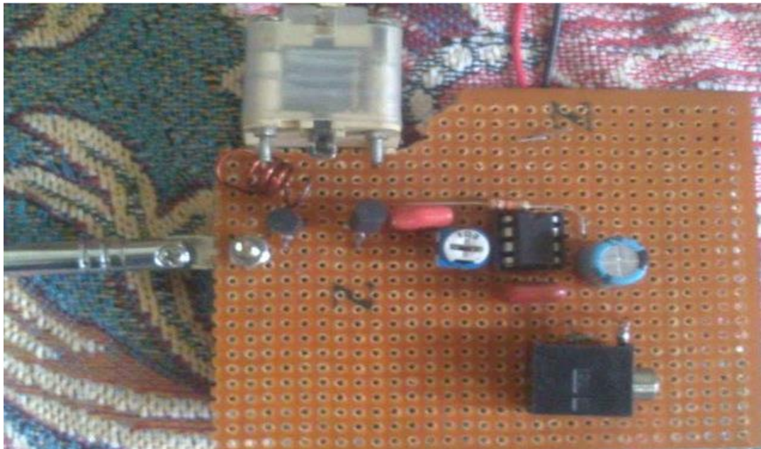
Figure GROUND STATION RECEIVER UNIT
