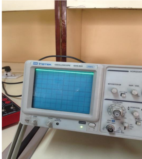
Figure 7.4. DEMODULATED OUTPUT WHEN INPUT IS 5 V
