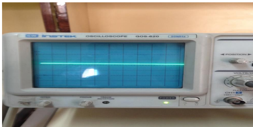
Figure 7.3. DEMODULATED OUTPUT WHEN INPUT IS 0 V
