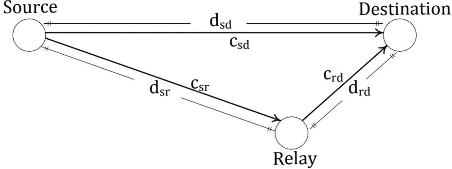
Figure 3.1: The relay channel.
