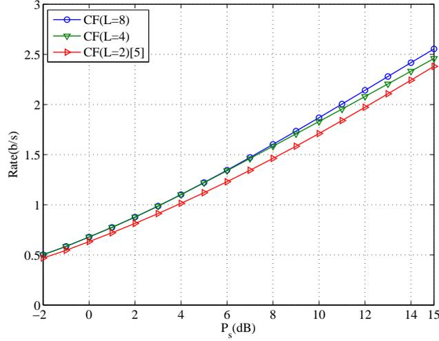
Figure 3.3: A comparison of CF achievable rates for several  $L$ . The parameters are set to  $M = 8$ ,  $P_r = -3$  dB,  $d_{rd} = 0.15$  m, and  $d_{sr} = 0.95$  m.
