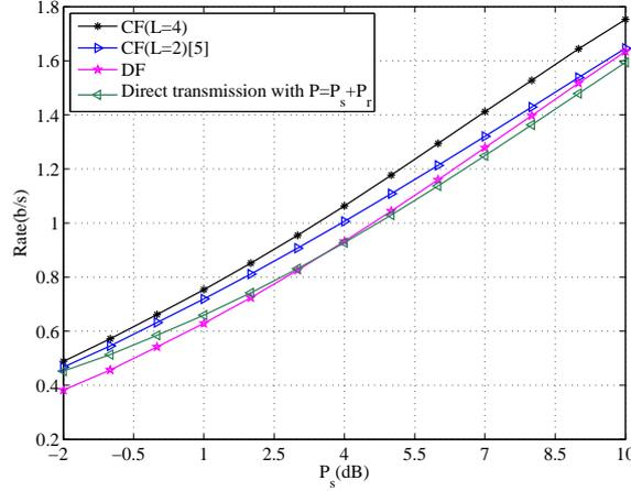
Figure 3.2: CF achievable rates versus the source power  $P_s$  for  $M = 4$  and their comparison with DF and direct transmission rates. The other parameters are set to  $P_r = -6$  dB,  $d_{rd} = 0.2$  m, and  $d_{sr} = 0.95$  m.
