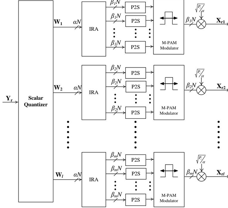
Figure 4.2: Multilevel DJSCC encoding at the relay using  $l$  IRA codes.
