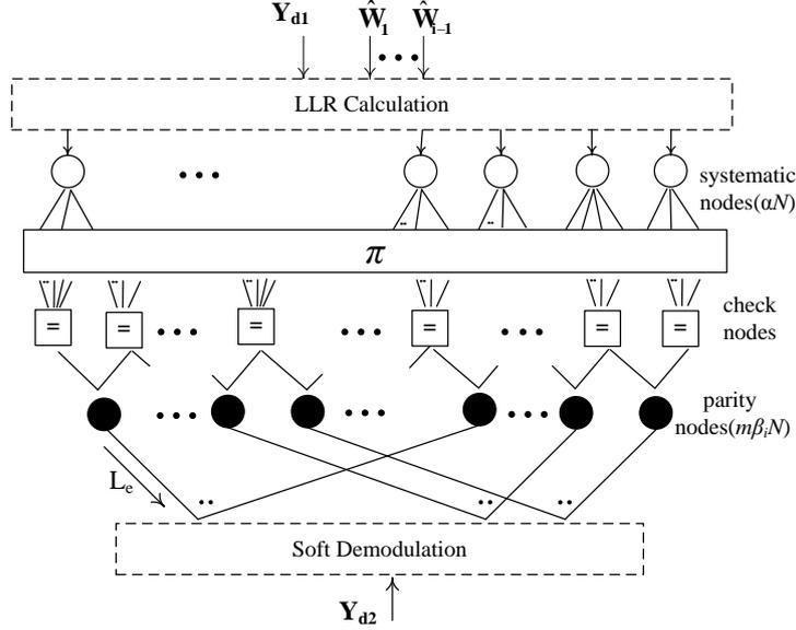
Figure 4.3: DJSCC decoder for the  $i$  –  $th$  quantization bit plane.
