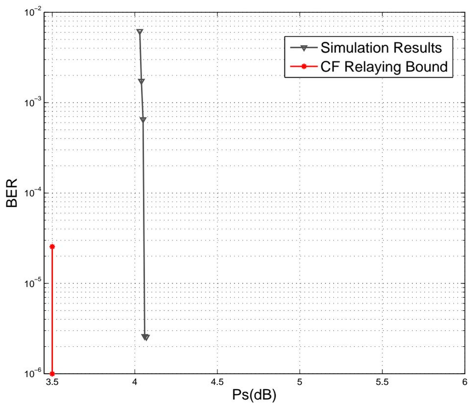
Figure 5.2: BER Vs. average source power  $P_s$  for an overall rate  $R_{CF} = 1(b/s)$ . Channel parameters are given Table 2.
