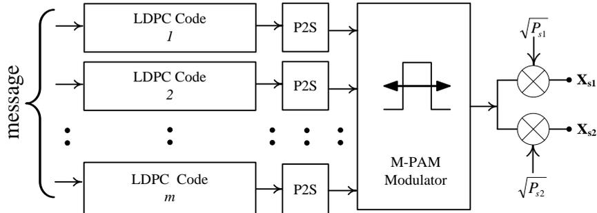
Figure 4.1: Encoding at the Source node using  $m$  LDPC codes. The P2S blocks indicate parallel to serial conversion.
