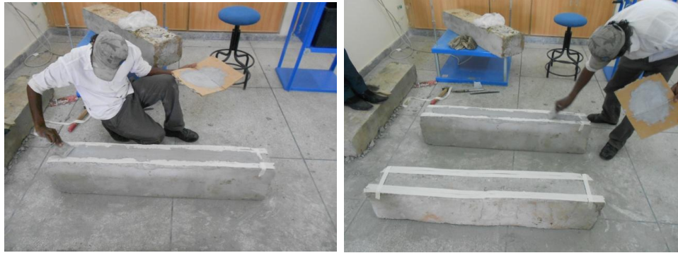
Figure 3-5: Applying Epoxy Resin
