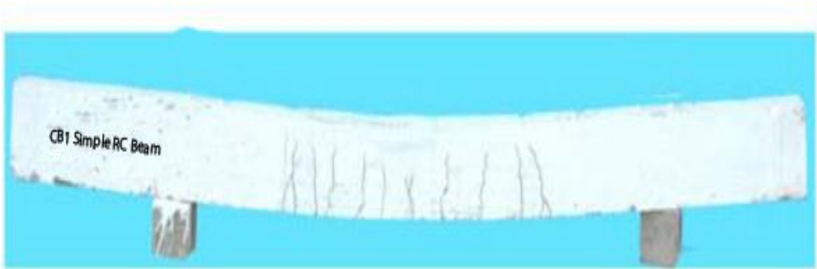
Figure 4-1: Cracking Pattern of RC Beam
