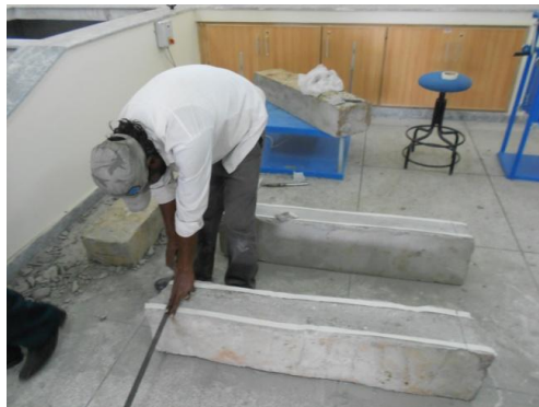
Figure 3-4: Preparing Beam and CFRP for epoxy
