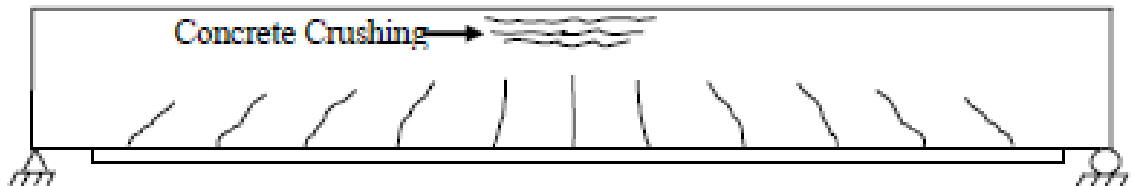
Figure 2-19: Crushing of compressive concrete
