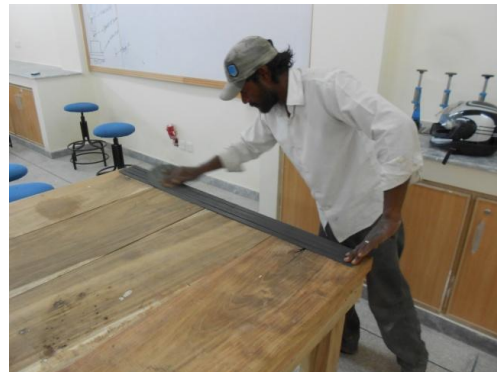
Figure 3-4: Preparing Beam and CFRP for epoxy
