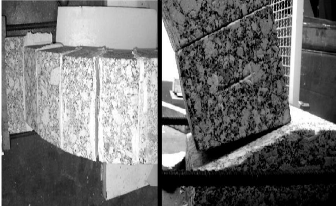
Figure 6.6 Hinges formed in experiment (1 rotational (left) + 1 sliding (right))
