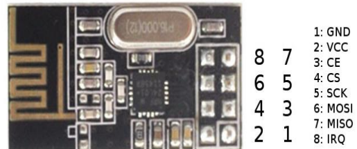
Figure 12 - nRF24I01 2.4 Ghz Module
