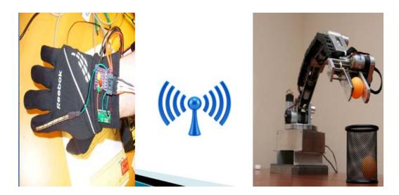
a. <u>Human hand with Glove.</u> This portion is designed with Glove on human hand which has flex resistors/ sensors on it. Here, when fingers are moved then flex sensors/ resistors convert the movement in voltage form which will be passed to controller (Arduino).
