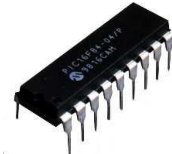
Figure 10: Programmable Interface Controller
