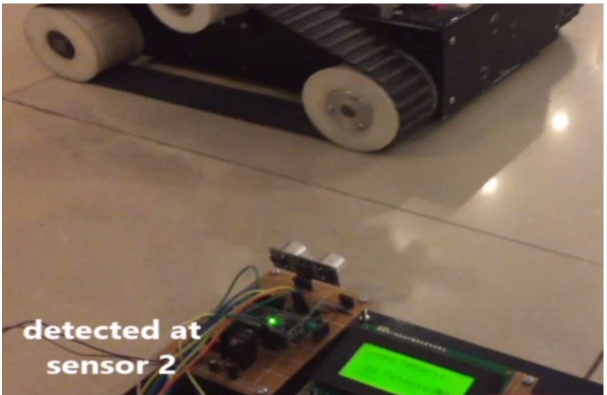
Fig 25: Vehicle Detected at Sensor 2
