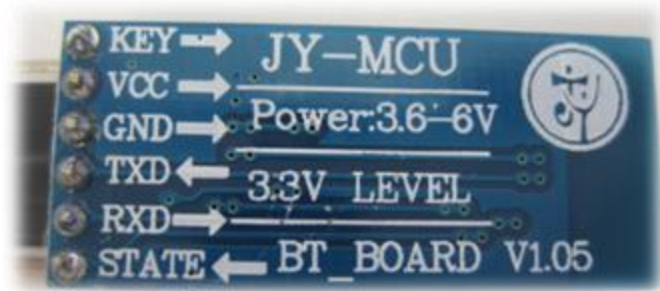
Figure 19: Bluetooth Pin Configuration
