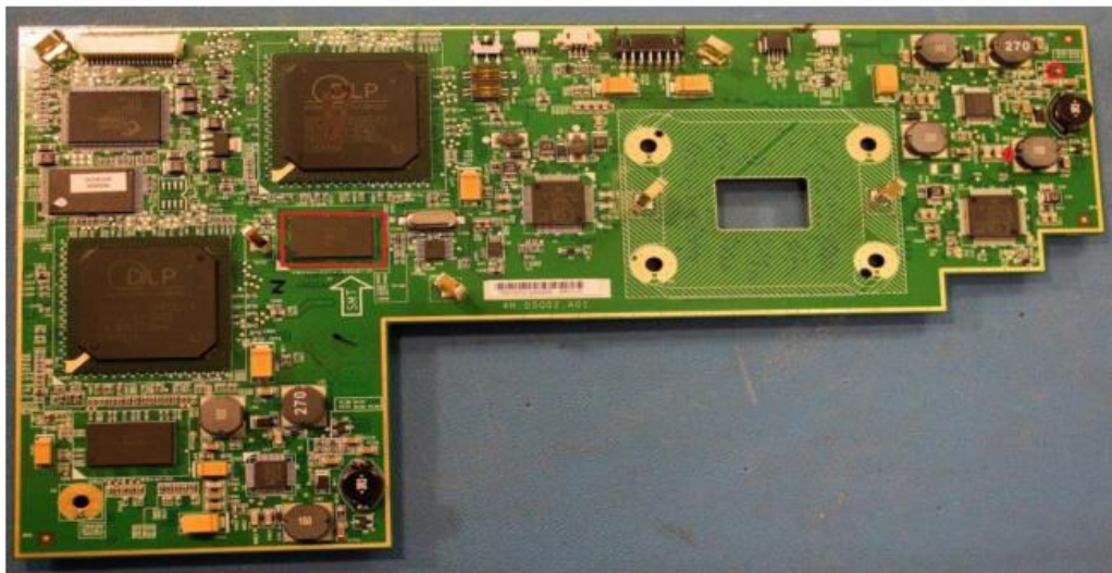
Figure 11 Internal view of a DLP projector having DLP technology from Texas Instruments
