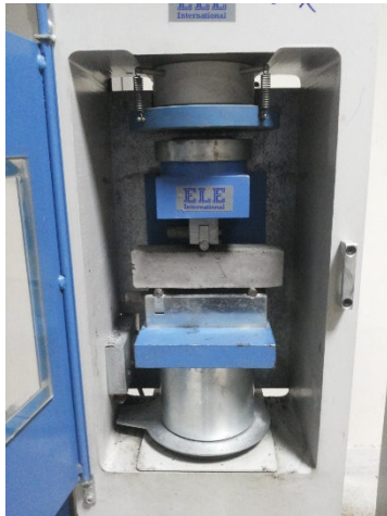
Figure 3.8 Dual Chamber for flexural and Compression test
