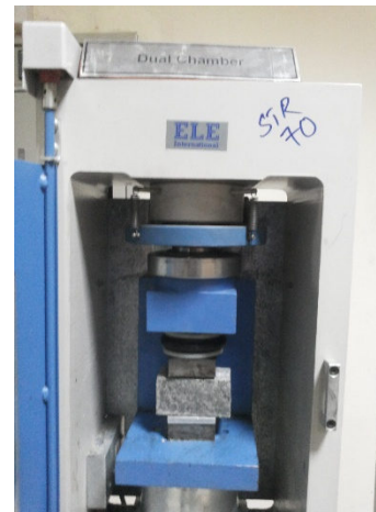
Figure 3.8 Dual Chamber for flexural and Compression test
