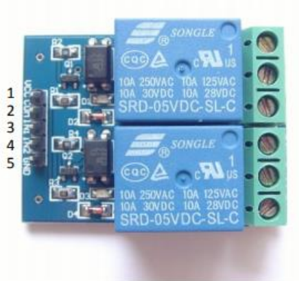
Figure 3-18: Pin Configuration of relay Module [26]
