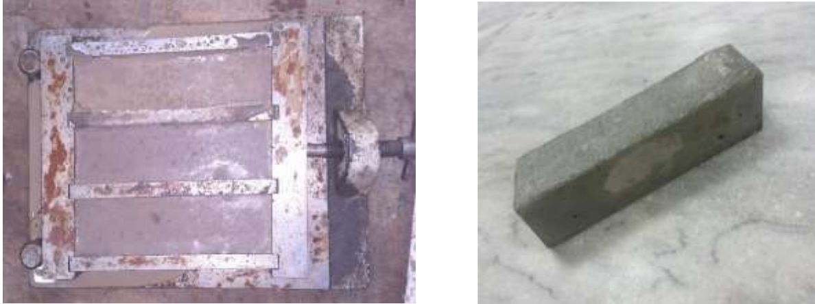
Figure 3: Casting molds and final shape of sample
