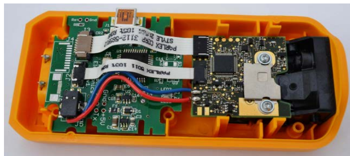
Figure D-1 Fluke 414D interfaced with Porcupine LR4 [17]
