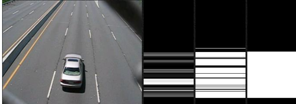
Figure 2 Background Subtraction as Car Enters
