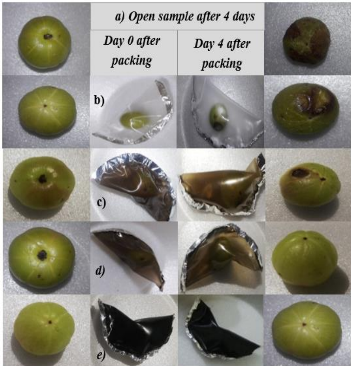
Figure 40 Images of packed fruit a) open b) PVA/St c) PVA/St/GO d) PVA/St/IrGO
