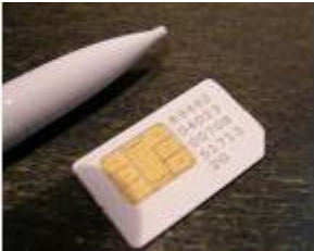
Fig 3-1: SIM card used in mobile phones, version 25x15 mm.
