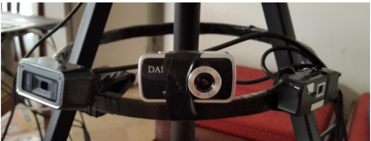
Figure 11: Actual Camera mount on tripod stand
