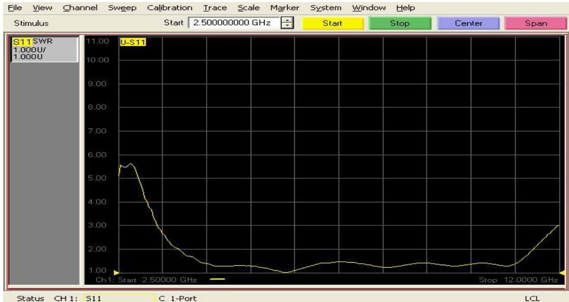
Figure-4.3: VNA Result for VSWR of Fabricated Design
