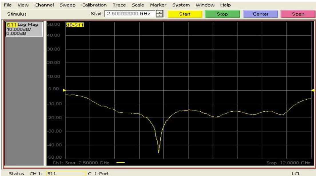
Figure-4.1: VNA Result for Return Loss of Fabricated Design
