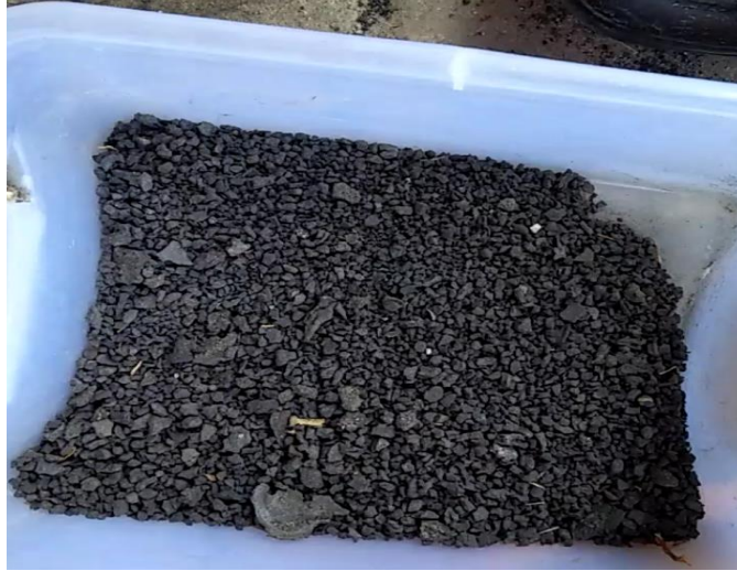
Figure 2: Dried and crushed SS taken from NUST waste water treatment plant
