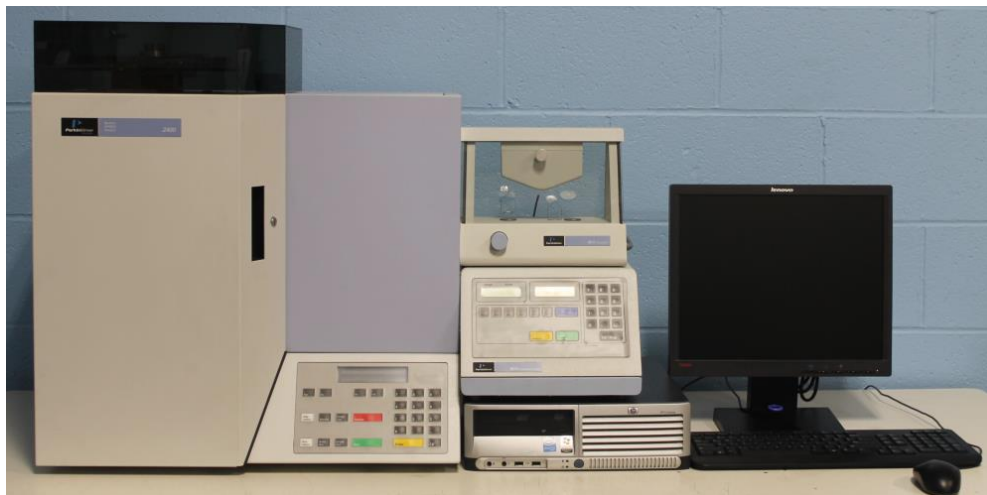
Figure 9: CHNS elemental analyzer (PerkinElmer 2400II, USA)
