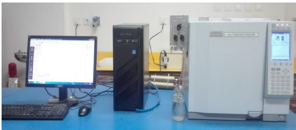
Figure 15: SHIMADZU GC-2010 plus gas chromatograph with TCD detector
