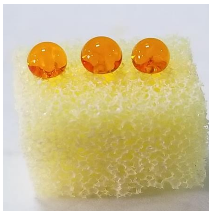
Figure 4. 21 Optical image of S1S1Z4S under excessive amount of water droplets (dyed orange)
