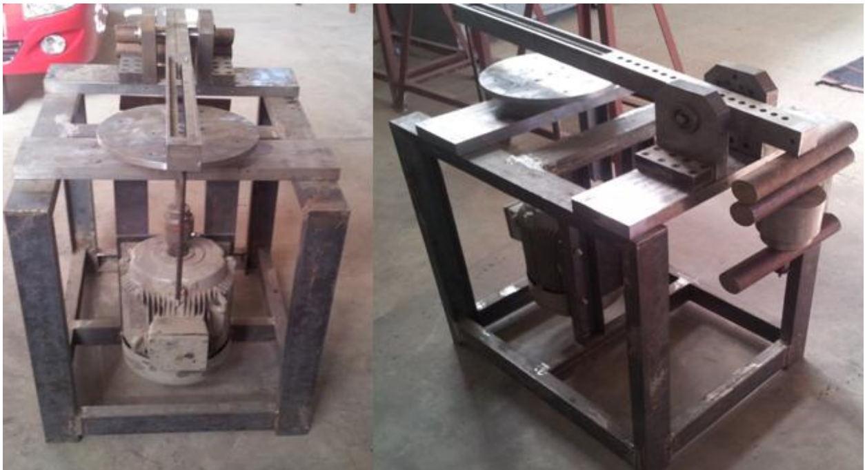
Figure 28 Indigenously fabricated pin-on-disk tribometer for tribological studies of hard-rock drilling
