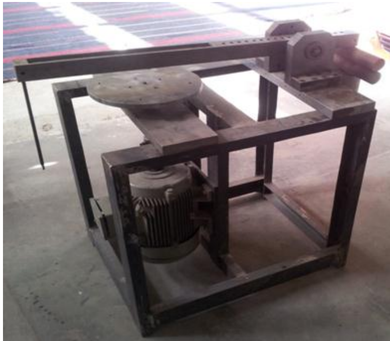
Figure 29 Side view of indigenously fabricated pin-on-disk tribometer for tribological studies of hard-rock drilling
