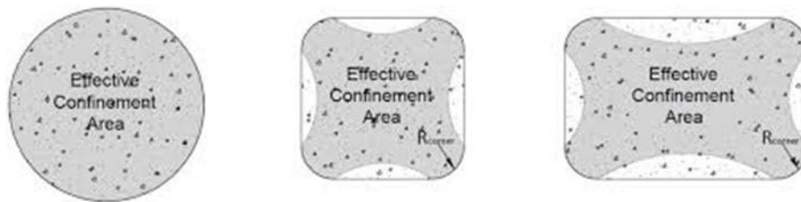
Figure 2. 10 Comparison of FRP-confinement in circular, square and rectangular columns. (Brighton & Parvin, 2014)
