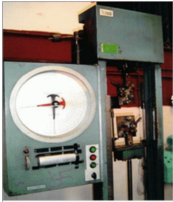
Figure 4. 4 Universal Testing Machine (UTM), Central Process Laboratory (Pakistan)
