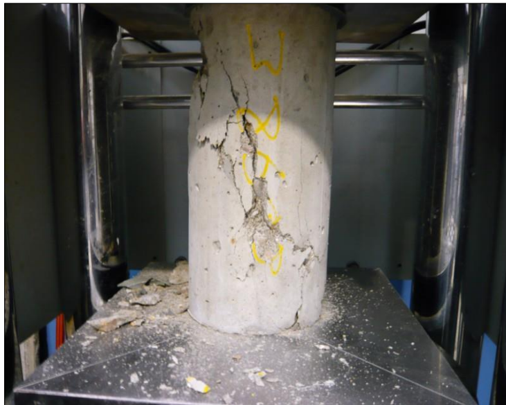
Figure 4. 3 Concrete Specimen Failures (UET, Peshawar)
