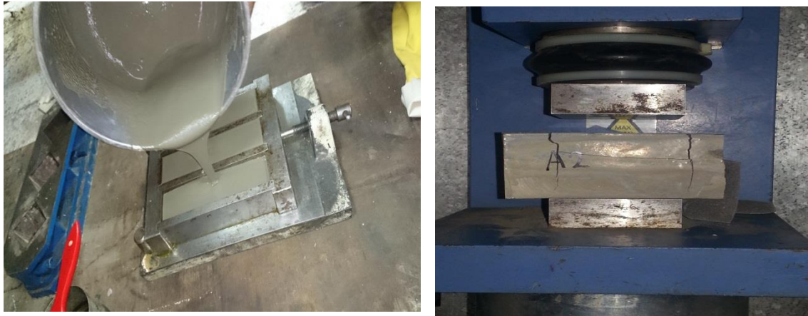
Figure 2.9.4: (left) Prism Molds, (right) Samples tested in Dual Chamber
