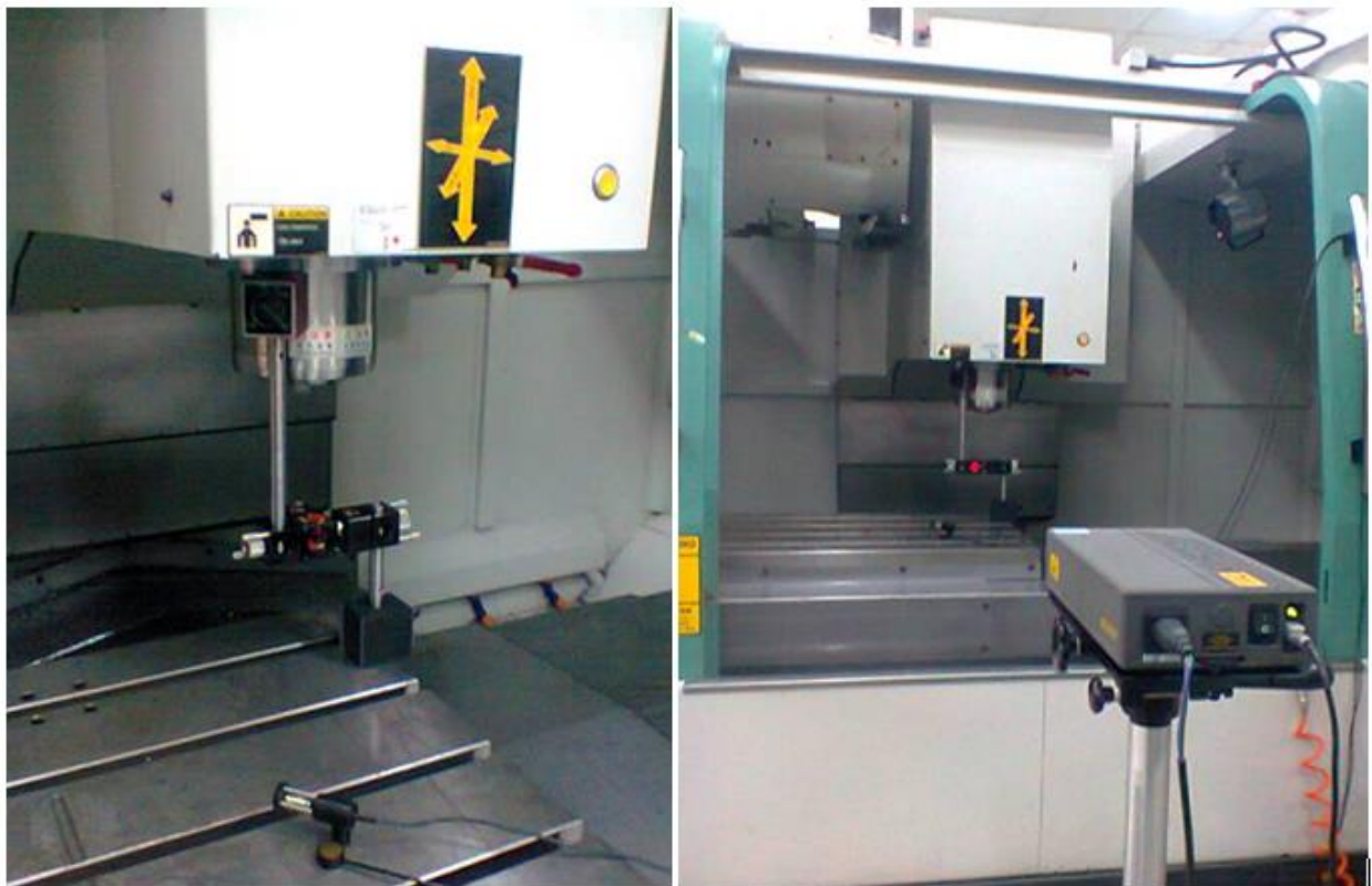
Figure 7.3 Laser Calibration of Machining Centre MV-1060 at SMME NUST
