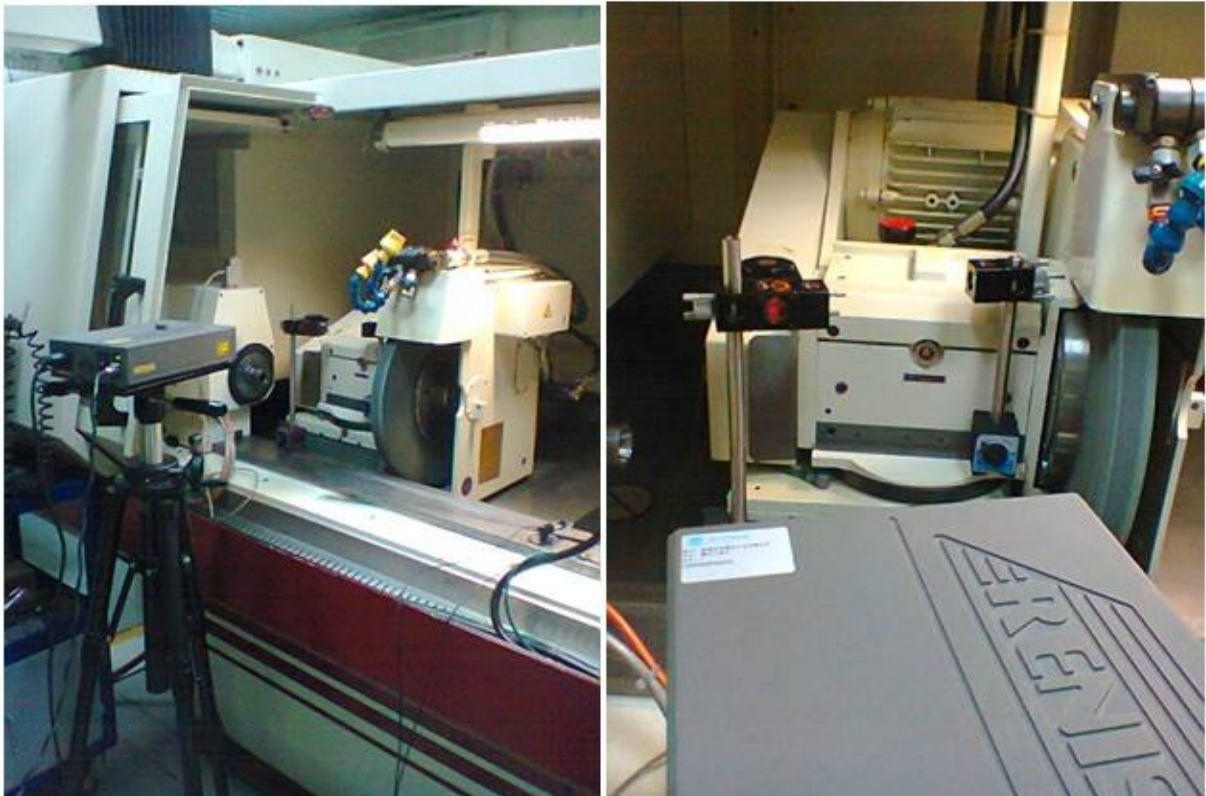
Figure 6.12 Laser setup for Diagonal measurement, Studer S-36
