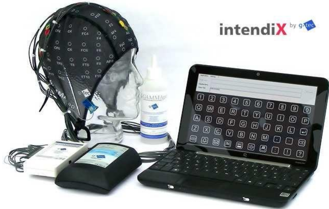
Figure 4 EEG signal acquisition system including electrodes cap, an amplifier and a monitor to see recorded signals [10]
