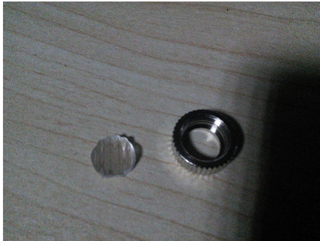
Figure 23 - Cylindrical Glass Lens with Screw Mount
