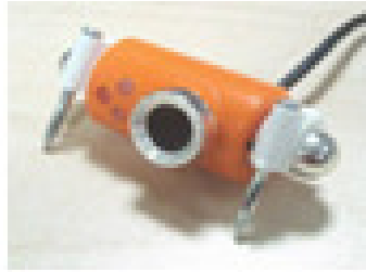
Figure 21 - VGA Camera Used In First Prototype
