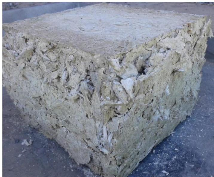
Figure 11: Fractured hempcrete specimen on subjection to compressive stress
