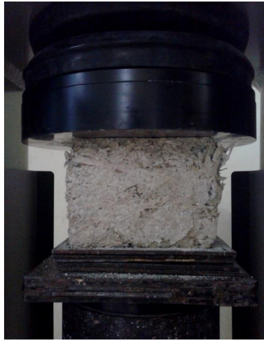
Figure 10: Hempcrete sample under applied stress
